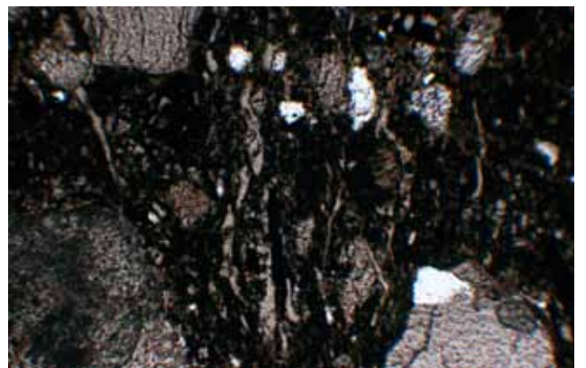
Fig. 6. Grave 121 vessel 2. Directional cracks in the ceramic body related to the vessel formation process. Polarizing microscope, one polarizer, 40x magnification.
