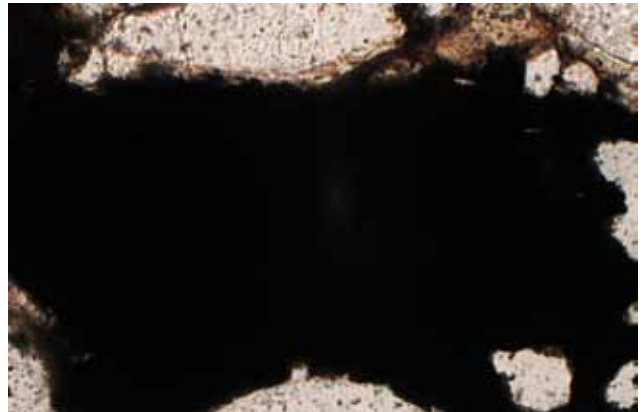
Fig. 17. Grave 135 vessel 2. Image of the cement composed mainly of tarry substance resembling wood tar. Polarizing microscope, one polarizer, 400x magnification
