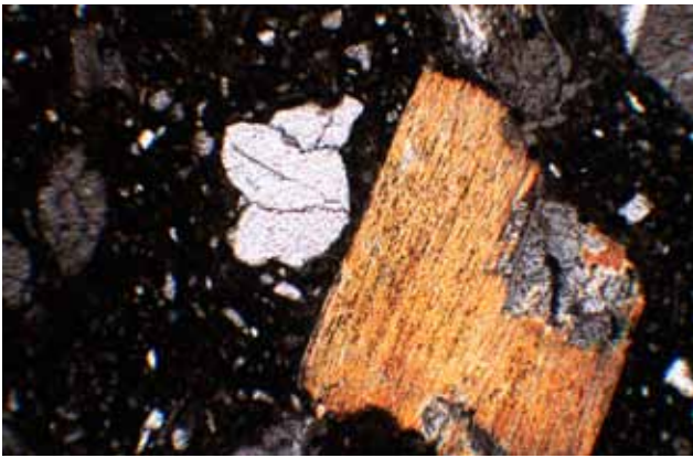
Fig. 7. Grave 121 vessel 3. A sheet of muscovite (white mica) embedded in the thermally altered ceramic body. Polarizing microscope, one polarizer, 40x magnification.
