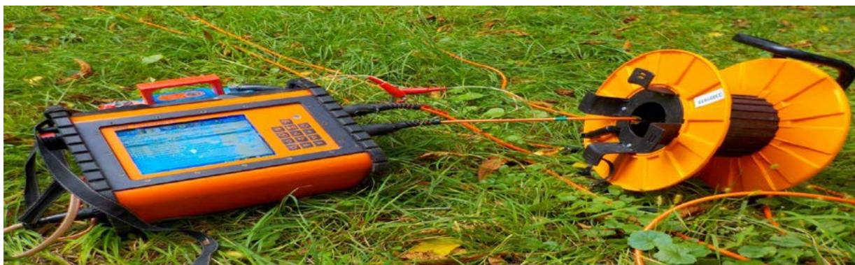
Ryc. 20. Aparatura do tomografii elektrooporowej TERRAMETER LS 8 kanałów (prod. ABEM, Szwecja). Fig. 20. Equipment for the electrical resistivity tomography TERRAMETER LS 8 channels (made by ABEM, Sweden).
