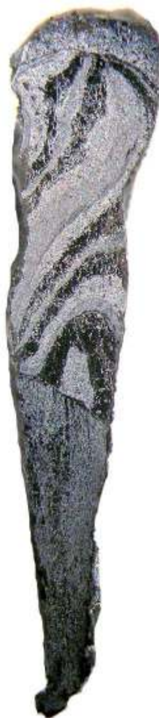
Fig. 294. Wrocław, Nowy Targ square, exca- vations 2010-2012. Knife, inv. no. 7397/11. Microscopic view of knife's cross-section after etching. Varied structures in different parts of the blade show its multi-material composition. Phot. B. Miazga
