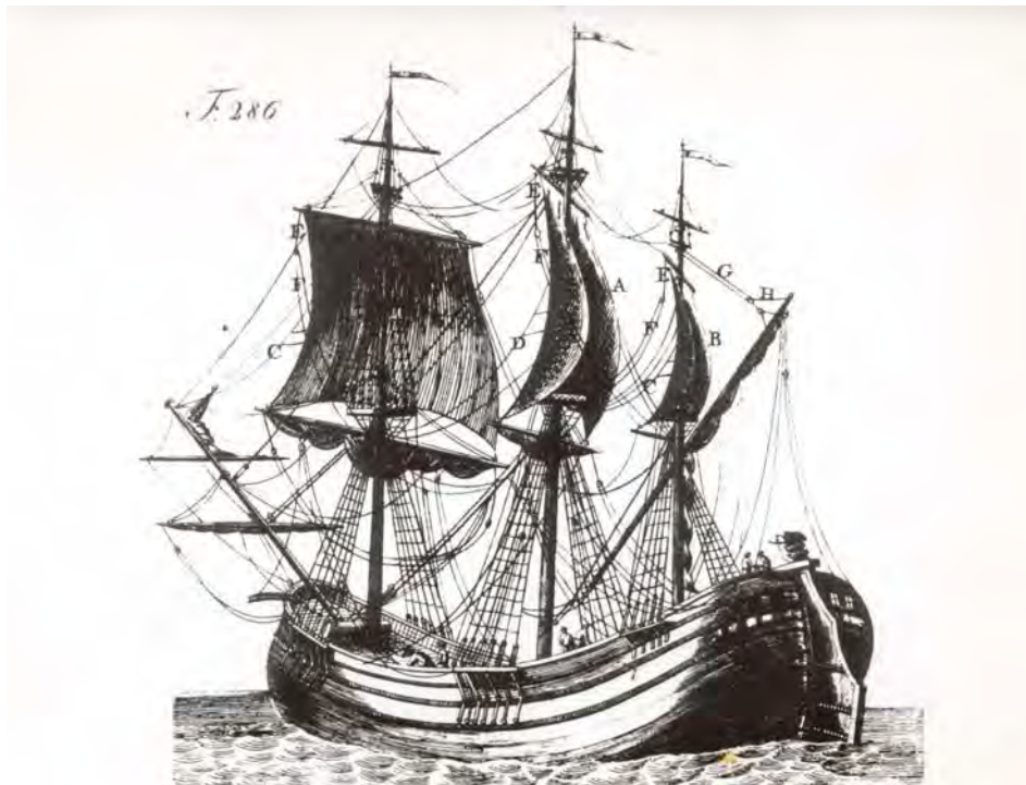
Fig. 7. A typical northern European cargo vessel – a galliot (drawing after J. H. Röding).
