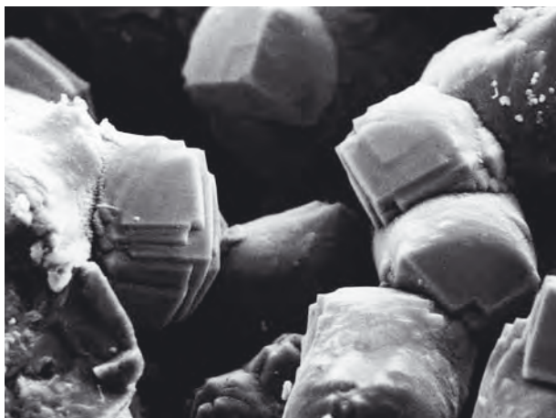
Fig. 11. Granular siderite at the stage of formation of crystallographic faces on individual grains. Scanning-microscope. Magn. x 2500 (photo by P. Dzierżanowski).
